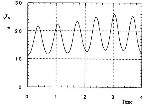
Fig. 9 Velocity norm trajectory of undamped NJM( $K_d=0$ )
