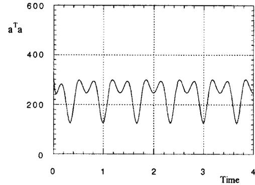
**Fig. 13** Acceleration norm trajectory of null space damped NJM( $K_d=5$ )
