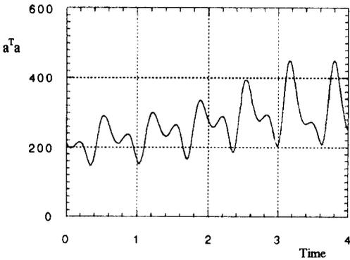
Fig. 10 Acceleration norm trajectory of undamped NJM( $K_d=0$ )
