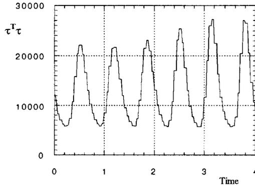
**Fig. 11** Torque norm trajectory of undamped NJM( $K_d=0$ )
