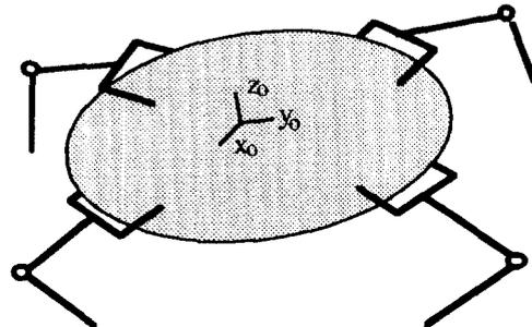
Fig. 1 Multiple cooperating redundant manipulators handling a common object
