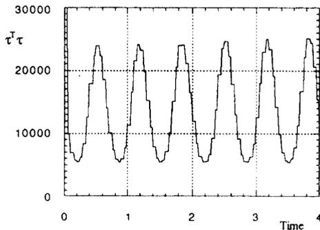
Fig. 8 Torque norm trajectory of null space damped JTM( $K_d=200$ )
