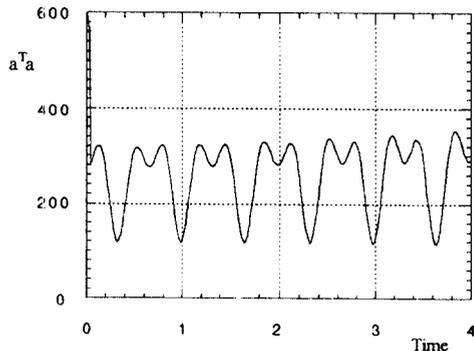
Fig. 7 Acceleration norm trajectory of null space damped JTM( $K_d=200$ )
