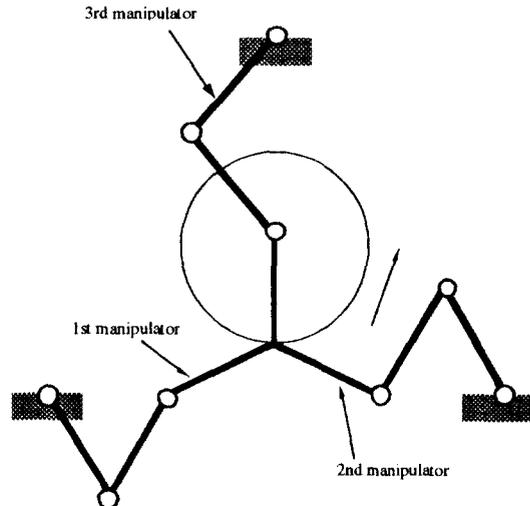
Fig. 2 Three cooperating redundant manipulators to the X-Y task space
