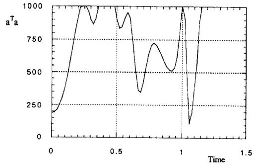
Fig. 4 Acceleration norm trajectory of undamped JTM( $K_d=0$ )
